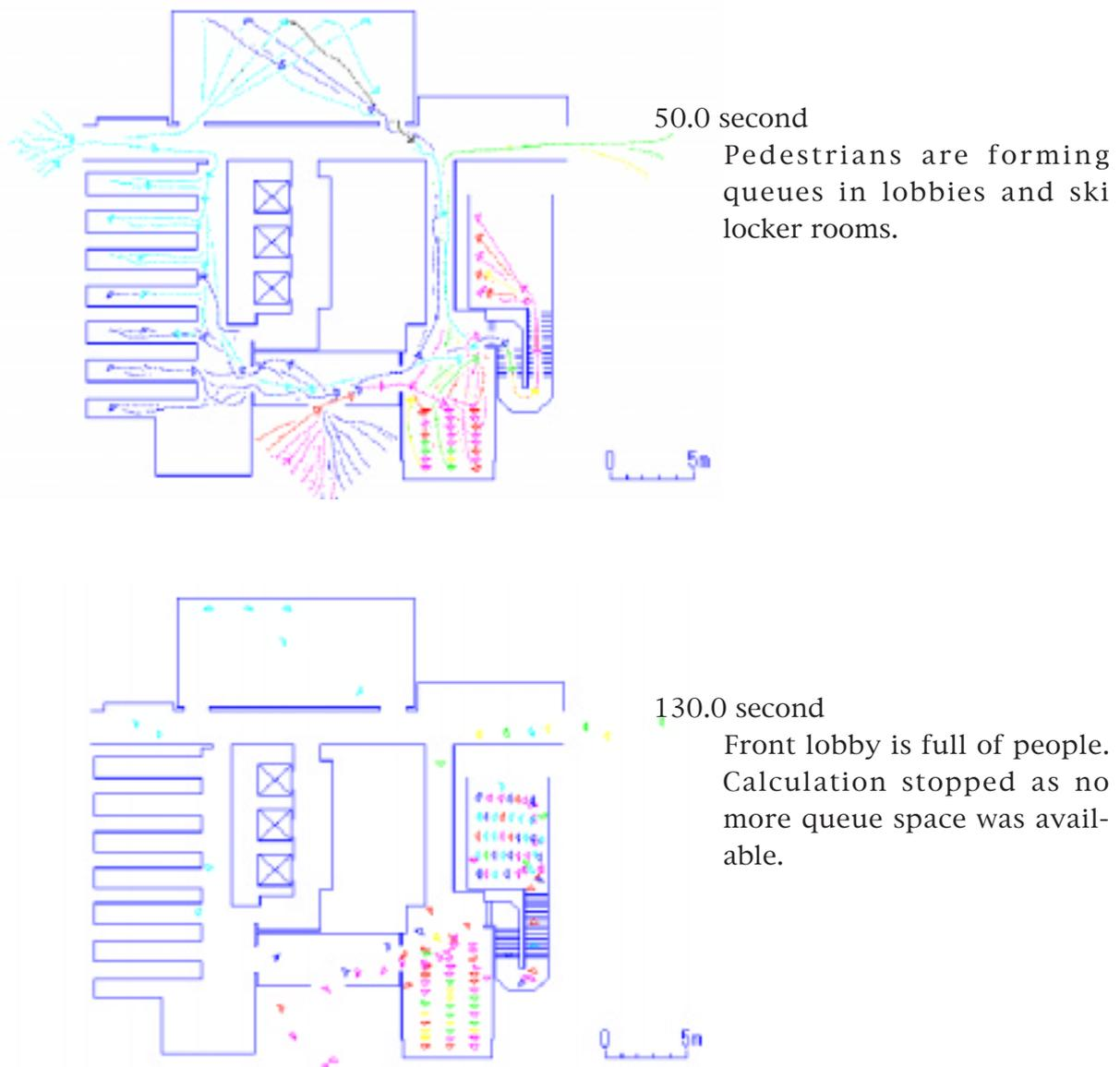
Figure 5. Simulation in the plan of a hotel
