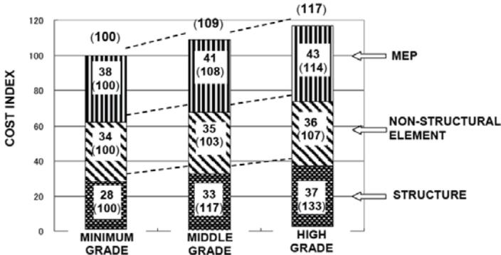
Fig. 2 : Seismic Performance Upgrading and Cost Increase
