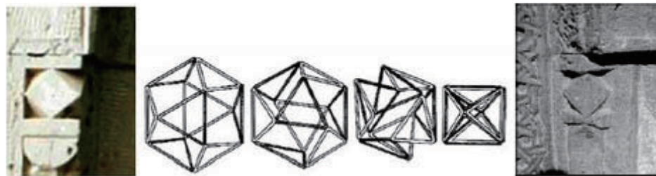
Fig. 10: “Jitterbug” representing the phase transformation between cuboctahedron and octahedron
