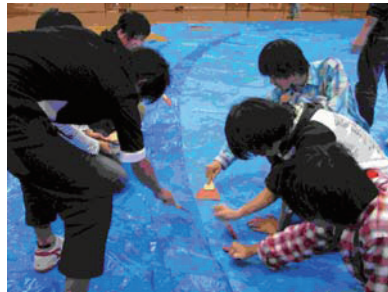
(2) Gluing for 25m diameter 2-D circular membrane bag
