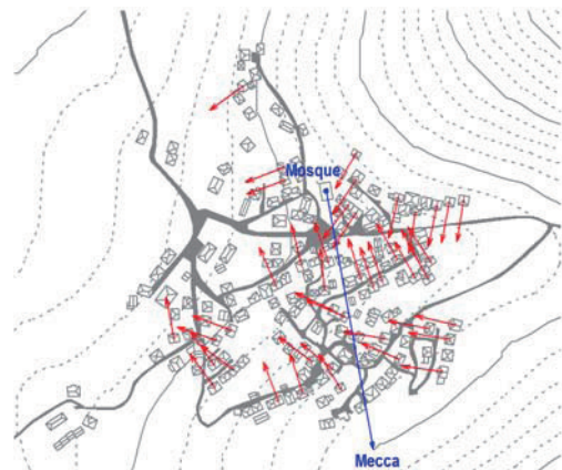
Fig. 25: Aspects of facades in Çiğdemlik Settlements 1:10,000
