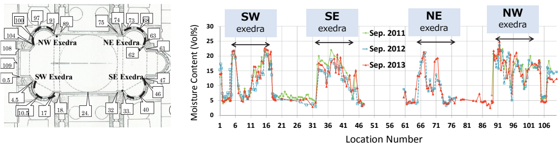
Fig. 2: The location numbers (Left) and moisture content of the inside walls measured at 2 nd Cornice level (Right)
