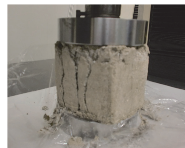
Fig. 4 Measurement of compressive strength of tataki cube
