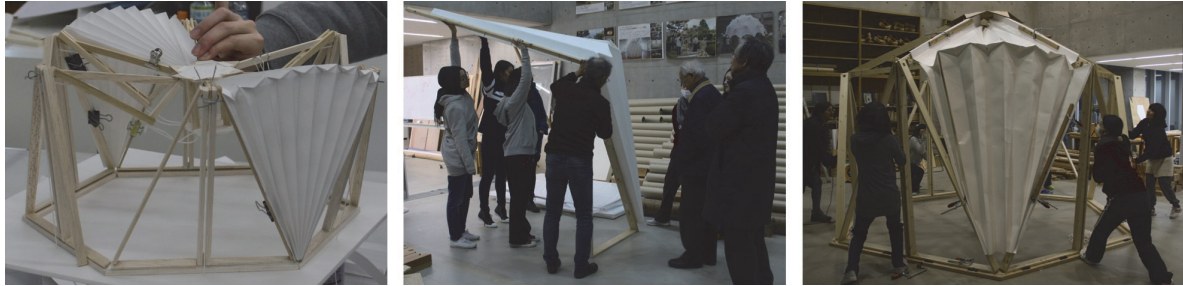
(a) 1:10 scaled model (b) Partial full-scale model (c) Entire full-scale model Fig. 6: Follow-up investigation of folded bellows to ensure full covering of the roof and walls
