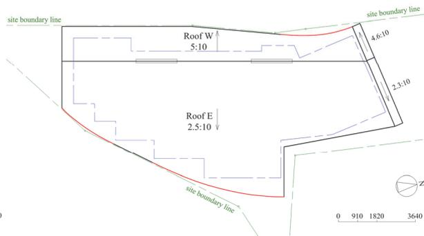
Fig. 3: Determined LAC  $C_W$  on the plane containing Roof W and LACs  $C_E$  and  $C_S$  on the plane containing Roof E S=1:250
