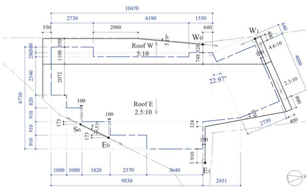
Fig. 2: Conditions of eaves on roof plan S=1:250
