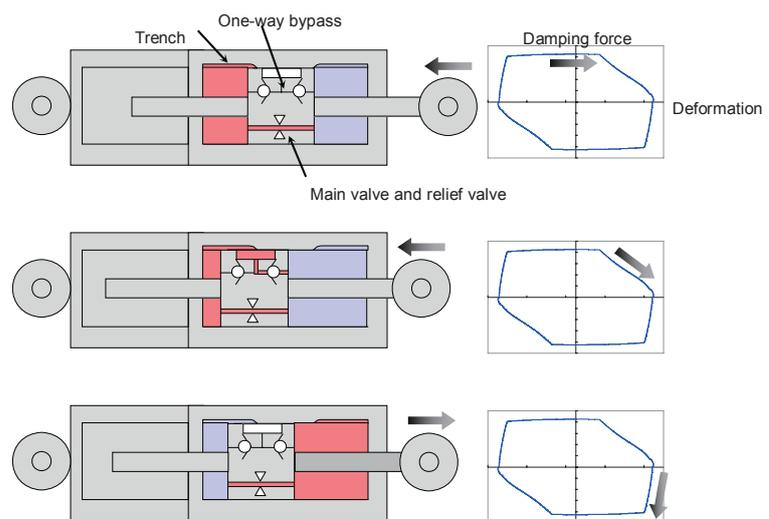
Fig. 2: Mechanism of a deformation-dependent oil damper
