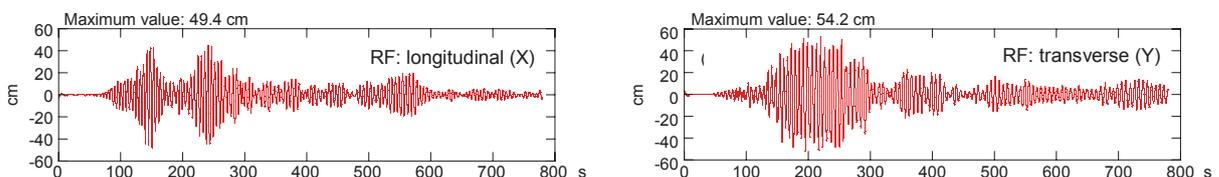
Fig. 9: Relative displacement waveform between RF and 1F
