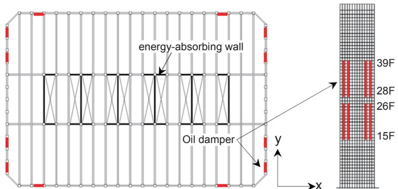
Fig. 4: Layout of oil dampers
