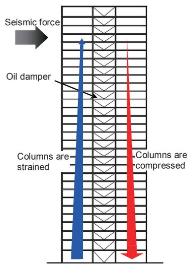
Fig. 1: Stress condition while seismic force is acting
