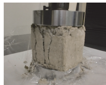
Fig. 4 Measurement of compressive strength of tataki cube
